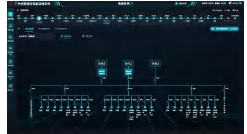
Distribution Cabinet Output Terminal Monitoring
